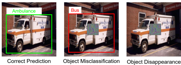
Figure 1: Illustration of a backdoor attack: On clean images, the network makes correct predictions. On images stamped with a trigger (enlarged here for better visualization), the network either misclassifies objects (Object Misclassification Attack), or does not detect objects at all (Object Disappearance Attack), depending on the attacker’s objective.
