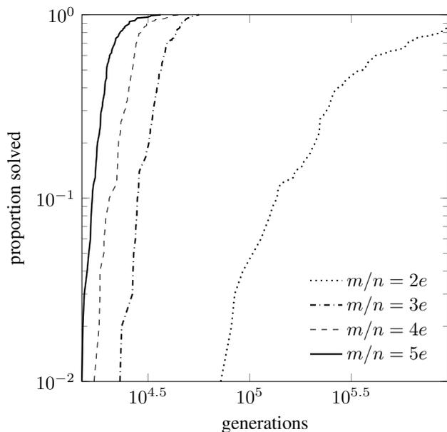
Figure 3: Empirical run length distributions on community attachment model, controlling for density. The curves are created by 100 runs of the (1+1) EA at each constraint density value  $m/n \in \{2e, 3e, 4e, 5e\}$ . Each formula contains  $n = 1000$  variables, community size  $s = 100$ , and localized clause probability  $p = 3/4$ .
