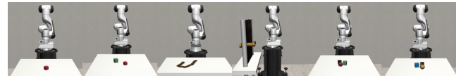
Figure 5: Manipulation tasks: Lift, Stack, Table Wiping, Door Opening, and two Stack Out-of-Distribution (OOD) variants. Stack OOD-A: add an interference term; Stack OOD-C: alter the block’s shape and color.
