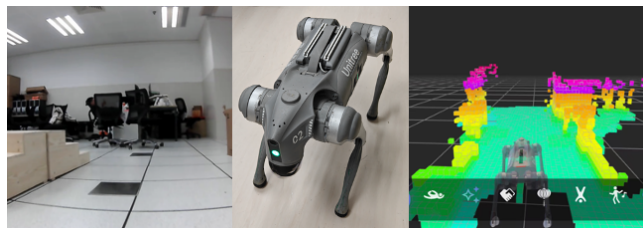
Figure 8: Navigation tasks tested in realistic indoor environments via Unitree Robotic Go2.
