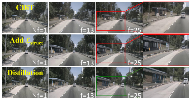
Figure 7: Ablation study. The first row shows CDiT predictions including lots of distortions, the second row adds the structure preservation term, and the last row shows the best.
