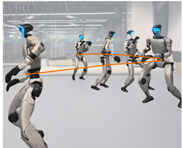
Figure 1: Snapshots of the humanoid robot executing whole-body trajectory tracking. WBC-SAP can track challenging dynamic trajectories over an extended duration, demonstrating that the SA2RT significantly improves the robustness of motion policies.
