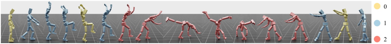
Figure 6: Visualization of expert activation throughout a cartwheel motion. Each frame is colored according to the number of active experts (yellow for 0, blue for 1, and red for 2). We observe that expert activation aligns with motion dynamics.
