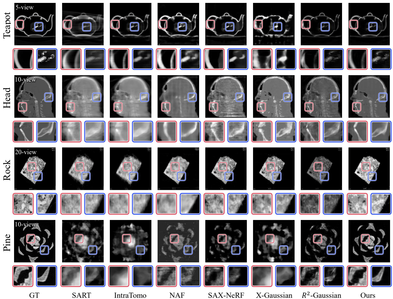
Figure 4: Qualitative comparisons of static CT reconstruction results across different view numbers (5, 10, and 20 views). Compared to SAX-NeRF and R^2 -Gaussian, our method consistently provides sharper structural details and fewer artifacts, especially under extremely sparse-view conditions.
