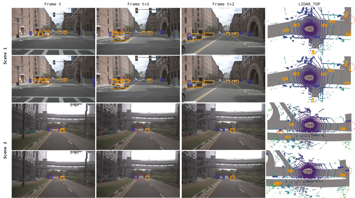
Figure 4: Qualitative results over three consecutive frames (front camera) in two scenes. The first and third row show the prediction made by the baseline model, while the second and fourth row demonstrate the predictive results of FTKD. In the last column, the LiDAR point cloud in BEV is display for frame t + 1 , except the last row (for t + 2 ) due to the limited BEV distance. FTKD successfully predicts an occluded car merging into the main road and a pedestrian crossing the street in the distance, highlighted by red dotted circles.
