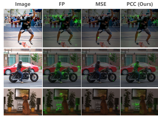
Figure 3: Attention heatmaps in the mask decoder with different quantization clipping methods. The distribution-aligned MSE leads to significant attention degradation, whereas our semantic-aligned PCC maintains the consistency with the FP model.
