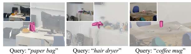
Figure 8: Open-vocabulary 3D object search. Given a text prompt, our method can accurately locate the corresponding object instances (pink) in a 3D scene.
