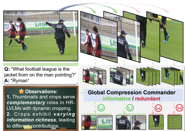
Figure 1: Design philosophy of “global-to-local” guided token compression. GlobalCom 2 evaluates the information richness of local crops from a global perspective to preserve informative regions while removing redundant ones.
