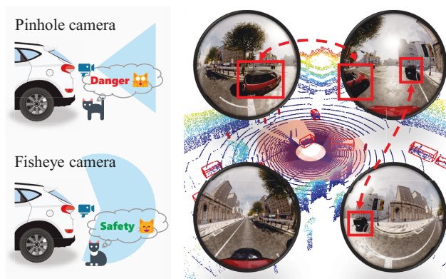
Figure 1: Left: The pinhole camera setup has blind spots in the near field, whereas the fisheye camera provides enhanced coverage for improved safety. Right: The same object is captured from multiple fisheye viewpoints.
