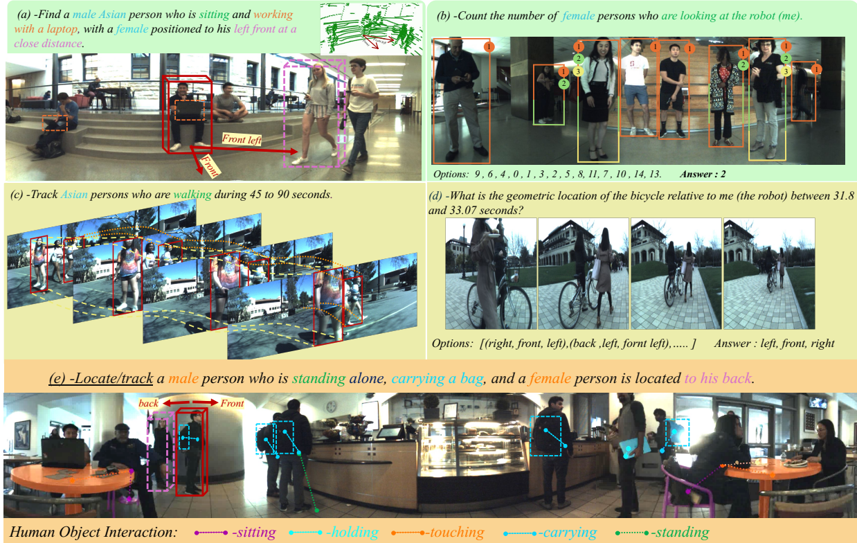
Figure 1: Illustration of JRDB-Reasoning on VG and VQA for images and videos. (a) and (e) depict VG tasks on images & HOI. (b) presents a VQA-Counting question with reasoning steps: (1) identify all humans, (2) filter for females, (3) find female looking at the robot. (c) illustrates a VG multi-object tracking task, while (d) shows a VQA-Wh question applied to a video.
