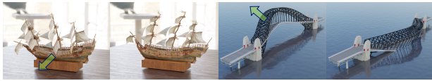
Figure 5: Experiments on high-resolution mesh objects. ElastoGen generates realistic nonlinear elastic dynamics under external forces. Both high-frequency local details and low-frequency global deformations are effectively captured with a carefully designed nested RNN architecture.
