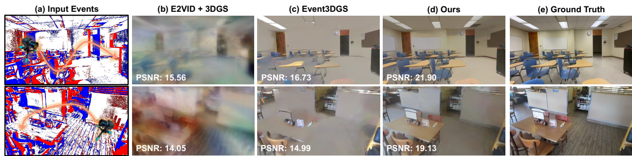
Figure 1: Comparison of Our EvDiff3D with baselines. Our EvDiff3D improves event-based 3DGS reconstruction by integrating event-based geometric constraints and an event-aware diffusion repair model.
