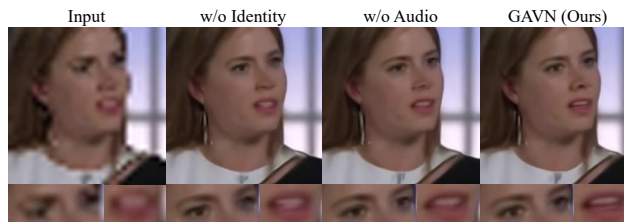
Figure 1: Restoration results of our proposed GAVN with and without identity features and audio signals. The frames reconstructed without using identity features and audio signals appear blurry in the left eye and tongue, respectively.
