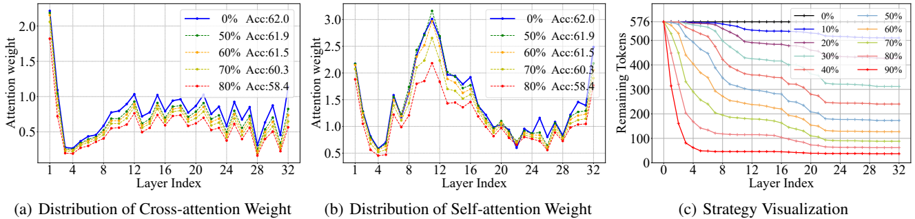
Figure 5: The visualization of impact of our FitPrune. (a) Distribution of cross-attention weights. (b) Distribution of self-attention weights. These distributions are based on LLaVA-1.5 7B for the GQA benchmark. (c) The number of tokens across the 32 layers under the different settings.
