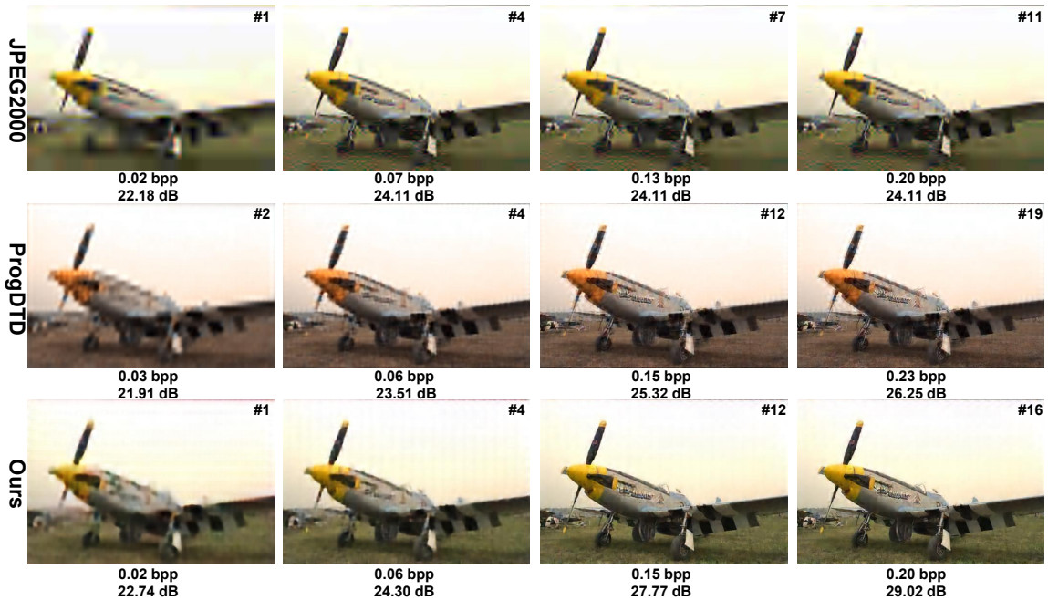
Figure 7: Visualizations of progressive coding under packet loss on Kodim20. #p denotes the reconstructed result after receiving the p-th packet at the decoder. The first column shows the initial results of progressive transmission without any packet loss for the three methods. The second column shows the results when the 3rd packet is lost. The third column shows the results when the 6th packet is also lost (for JPEG2000, only the 3rd packet is lost). The fourth column shows the decoded results after the progressive transmission is completed with packet loss. Our method consistently demonstrates superior performance.
