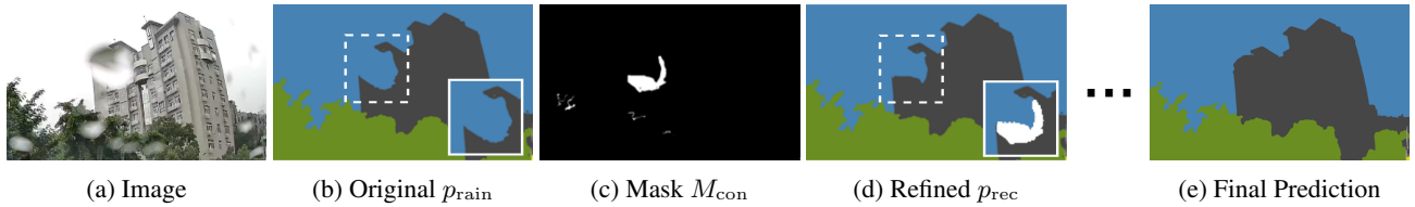
Figure 3: The illustration of the mask-based raindrop recovery in one iteration. In (b), the pseudo-labels are misled by raindrops. In the second round, upon inputting the masked image into the network, we rectify the wrong pseudo-labels by employing the confidence mask, as illustrated in (c). This process aims to correct the erroneous pseudo-labels that were influenced by raindrops, shown in (d). Over many iterations, the entire erroneous region will be filled, resulting in the final prediction in (e).
