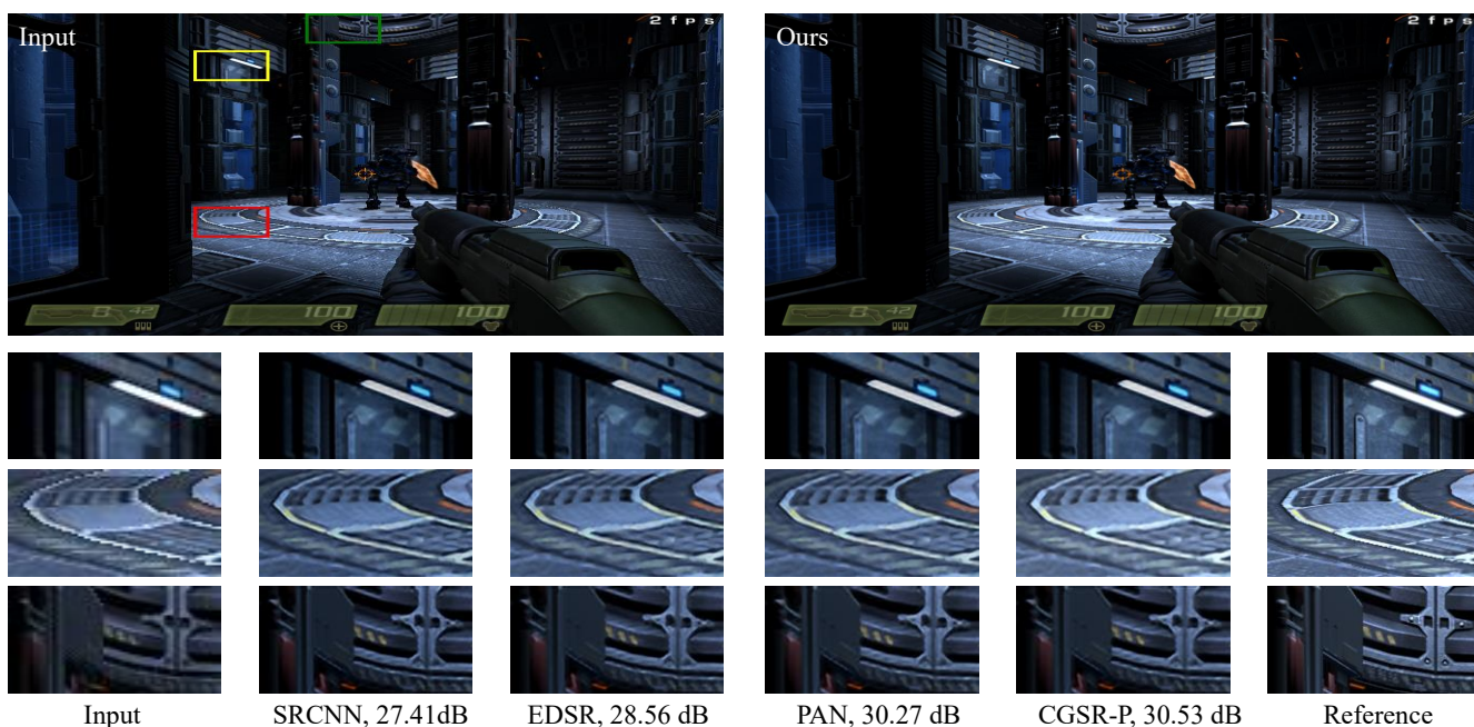
Figure 5: Visual results of the CGSR-P versus various SR networks on the Quake 4 trace.
