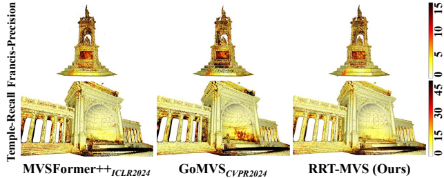
Figure 7: Qualitative comparisons of point clouds with top-2 published methods (Cao, Ren, and Fu 2024; Wu et al. 2024) on the Tanks-and-Temples benchmark. Brighter areas indicate smaller errors with distance threshold [ mm ].
