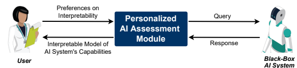
Figure 1: The personalized AI assessment module uses the user’s preferred vocabulary, queries the AI system, and delivers an interpretable model of the AI system’s capabilities.
