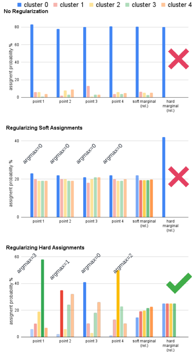
Figure 1: Top: with no regularization, the model collapses. Middle: soft regularization encourages uniform soft assignments but the argmax is constant. Bottom: hard regularization causes the argmax to change, and avoids collapse.
