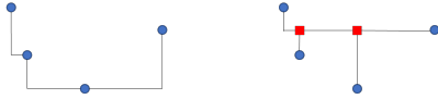
Figure 1: (L) Rectilinear spanning tree of input (blue) points. (R) Rectilinear Steiner minimum tree (red points are Steiner points).
