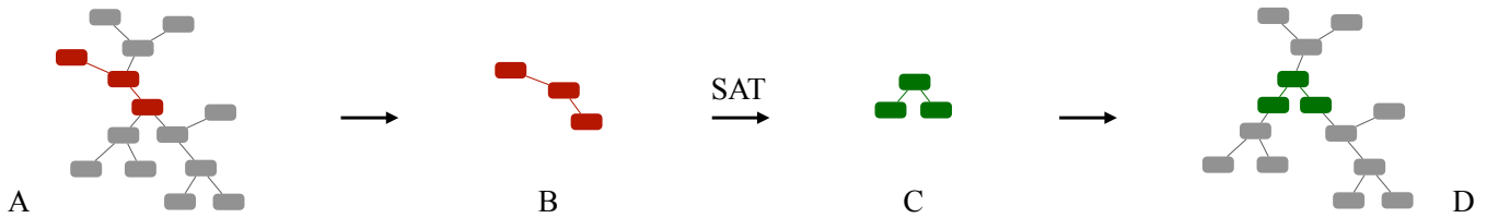
Figure 1: One single SAT-based improvement step within TW-SLIM. From A to B: a subtree that induces a local instance whose size does not exceed the local budget is selected; from B to C: an improved tree decomposition for the local instance is computed with a SAT call; from C to D, the original subtree is replaced by an improved subtree according to replacement consistency properties.
