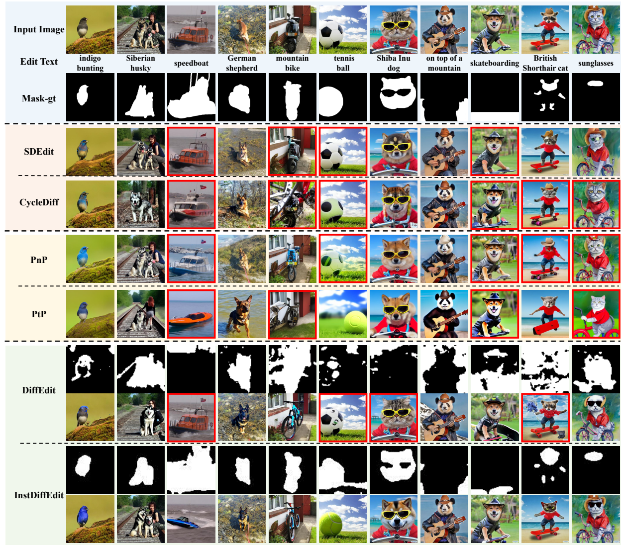
Figure 6: Visualizations of the generated masks and edited images of InstDiffEdit and the compared methods. Compared with DiffEdit, the masks of InstDiffEdit are closer to the human-labeled ones. Moreover, the comparisons with the latent-based and attention-based approaches also show the merit of the instant mask in our InstDiffEdit. The red boxes refers to failed editions.
