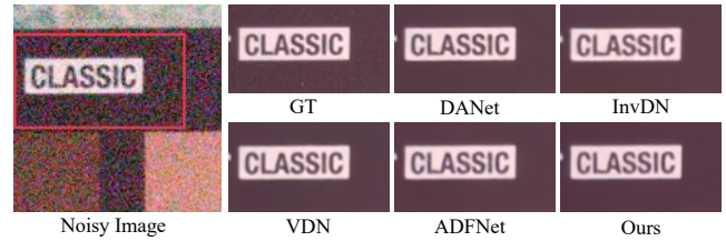
Figure 6: Visual comparison of LIDFormer with other efficient and lightweight denoising methods on SIDD.
