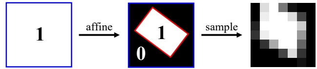
Figure 3: The translation between the predicted bounding box and the activation mask after affine transformation. The blue box represents the proposal region and the red box represents the activation mask.
