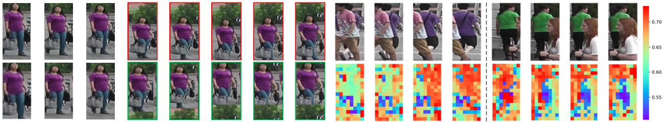
(a) Visualization of Filter-based Patch Alignment. The first row is an example of misaligned videos, while the second is the video sequence after alignment. (b) Visualization of Correlation Attention. The first row is two examples of videos under occlusion, while the second is the corresponding temporal correlation s_t .
