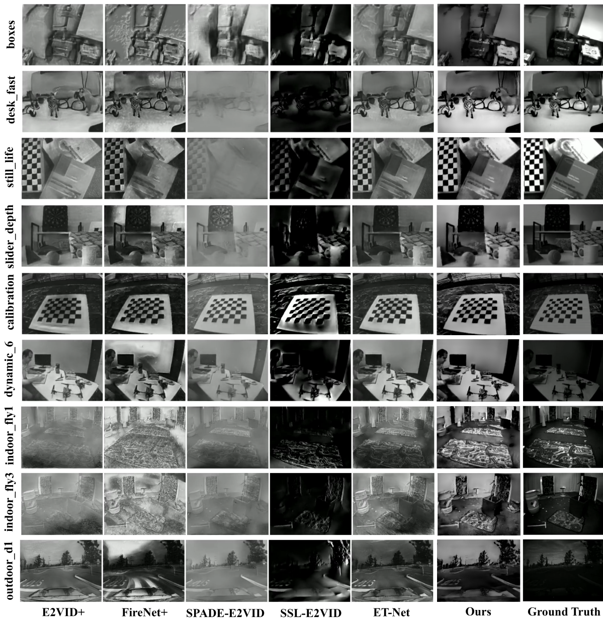
Figure 5: Qualitative Analysis across Datasets. Comparative visualizations of sequence data from HQF (rows 1-3), IJRR (rows 4-6), and MVSEC (rows 7-9). The evaluated baseline methods often exhibit limitations such as diminished contrast, noticeable blur, and prominent artifacts. In contrast, our reconstructions offer high contrast and are adept at maintaining sharp edge details, while manifesting minimal artifacts in regions devoid of texture.
