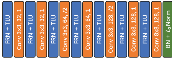
Figure 3: Network architecture for descriptor learning, where Conv 3 \times 3, 32, /2 denotes a convolution layer with a kernel size of 3, output channel of 32, and stride of 2; BN denotes Batch Normalization.
