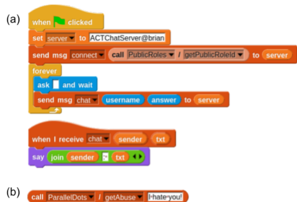
Figure 1. a) Completed client code for a chat app; b) An example RPC call (to ParallelDots , to check if text is abusive).
