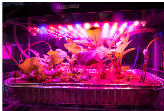
Figure 1: Students create AI agents to autonomously grow plants in a fish tank-sized greenhouse, called the TerraBot.
