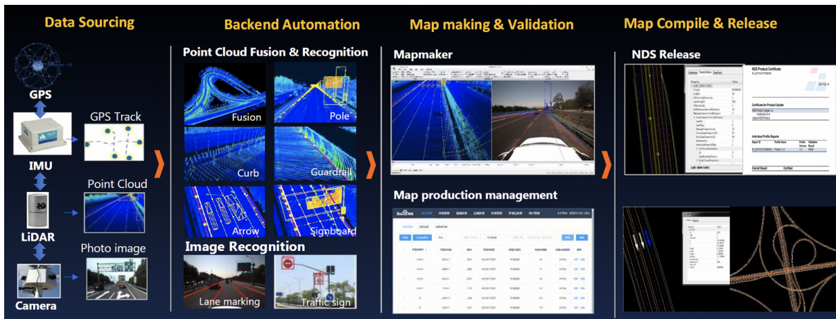
Figure 1: Basic production process of HD maps: (1) Data sourcing; (2) Backend Automation; (3) Map making and validation; (4) Map compile and release. Example shown uses the Baidu Apollo HD Map production (Ma 2018).
