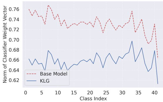
Figure 4: The norm of the classifier weight vector for each class. The class indexes are sorted by the number of samples (head to tail). We exclude the 'No Relation' to better view the trend. We can observe that KLG has similar vector norms across all classes.
