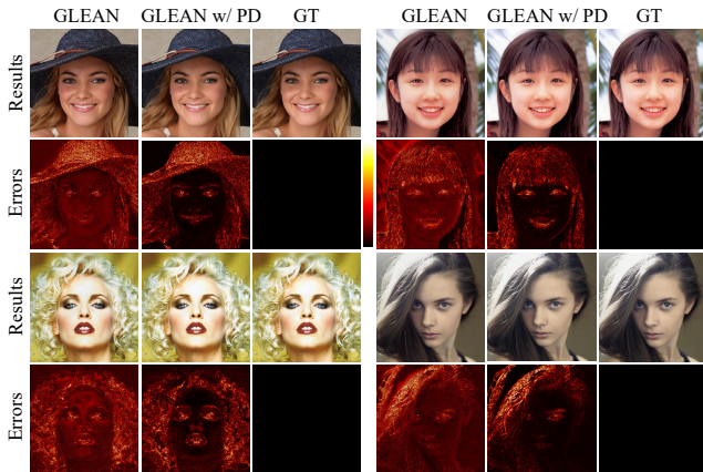
Figure 4: Qualitative results on 8\times face SR. GLEAN yields high-quality results. However, it still suffers low-frequency inconsistencies, e.g., inconsistent structures and colors in lips, eyes, and large areas of skin color deviations. The use of PD helps eliminate all the low-frequency inconsistencies, as can be clearly observed from the error maps.
