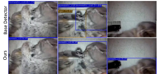
Figure 1: These frames suffer from various degradation, like motion blur and occlusion, making the base detector YOLOX fail to accurately detect the objects, while our method could.
