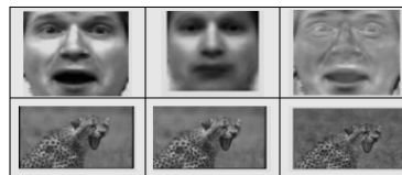
Figure 1: The left image in each row is the original data, the middle is the low rank part while the right one is the residual part. Our goal is to preserve those discriminative edges by finding robust image projections from low-rank residuals.
