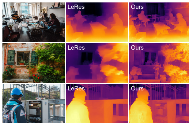
Figure 1: We propose a multi-resolution depth map fusion method to recover high-resolution depth maps. Compared with the single-resolution depth estimation network, the proposed method recovers wide levels of details.
