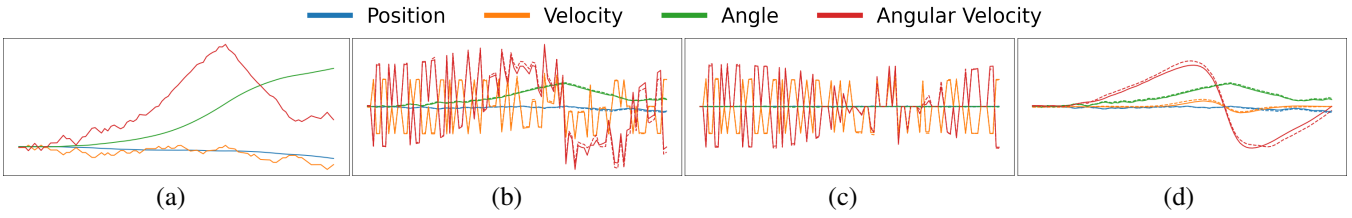
Figure 4: Disentangling refference and exafference in Cartpole. Observations and (estimated) effects are shown over time, with the agent taking an action at each step. Graphs show (a) observation, (b) total effects, (c) refferent effects, and (d) exafferent effects. Estimated effects are shown as dotted lines. An action is an instantaneous force applied to the cart which has an instantaneous effect on the carts (angular) velocity. Actions do not have an instantaneous effect on the carts position or angle.
