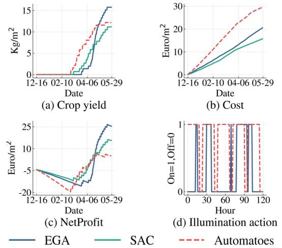
Figure 4: Performance comparison of different methods on our incremental simulator. (a)-(c) denote economic effectiveness simulated by different methods; (d) shows the 120-hour illumination action provided by EGA and *Automatoes*.
