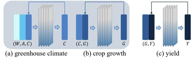
Figure 2: Network structure of the incremental simulator. (a) and (b) represent the greenhouse climate module and the crop growth module, respectively, which simulate the greenhouse planting process at hourly level. (c) represents the yield module, which simulates at daily level.
