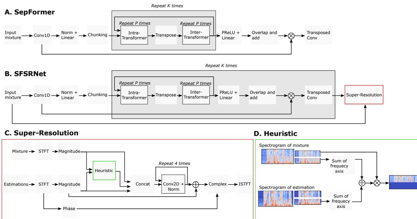
Figure 3: Comparison with previous SOTA (A) and the SFSRNet architecture (B).
