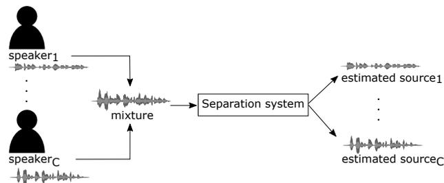
Figure 1: Single-channel audio source separation.
