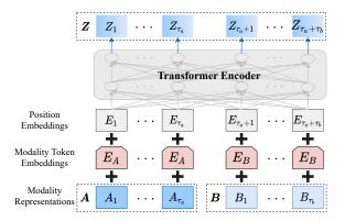
Figure 3: Structure of Cross-Modal Encoder (CME) between two modalities **A** and **B**. The two input modality representations, modality token embeddings and position embeddings are summed and fed into the Transformer encoder.
