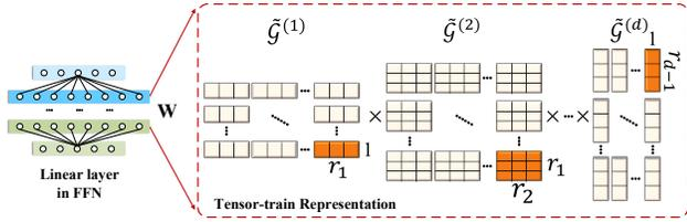
Figure 2: Tensor-train decomposition of weight matrix  $\mathbf{W}$  in the feed forward networks.
