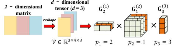
Figure 1: A 2-way weight matrix example for tensor-train decomposition.
