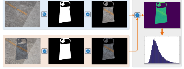
Figure 2: A simplified representation of one pair shadow images statistical analysis from the ISTD dataset. We find the ratio map \mathbf{R} is not uniform distribution in the umbra areas, which shows the shadow image’s spatially-variant property in the umbra region. Thus, applying a uniform transformation (e.g., Eqn. (6)) for all pixels in the umbra area is inaccurate. (Best viewed on-screen.)
