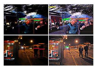
Figure 4: Detection results of YOLOv3 II (left column) and our IA-YOLO (right column) on synthetic VOC\_Dark\_test images (top row) and real-world ExDark low-light images (bottom row). The proposed method learns to enhance the image contrast with more details.
