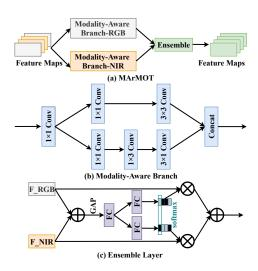
Figure 2: Details of MArMOT. The BN+ReLU layers after each Conv layer and the ReLU layers after each FC layer are omitted for clarity. Herein, ⊕ and ⊗ denote the operations of element-wise addition and multiplication respectively. F\_RGB and F\_NIR denote the output features of RGB and NIR after two parallel modality-aware branches respectively. GAP indicates the global average pooling.
