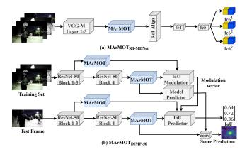
Figure 4: Visualization of the tracking architectures with MArMOT. (a) and (b) show the detailed structures of MArMOT combining with RT-MDNet and DiMP-50.
