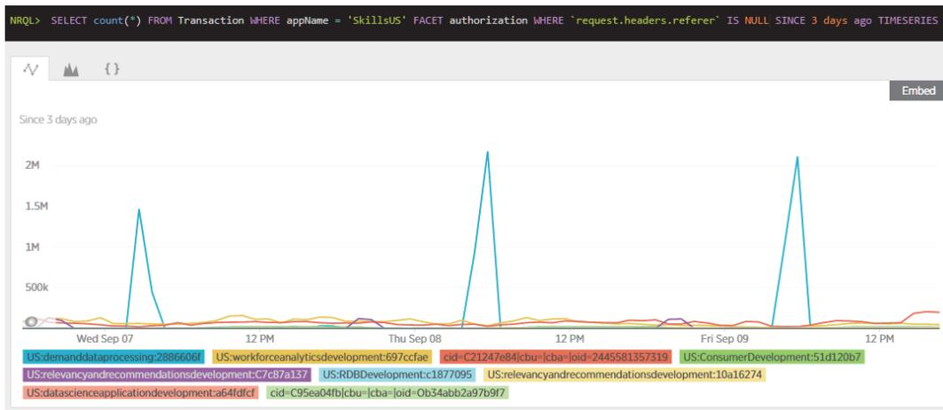
Figure 4: Number of Requests per Client ID over the last three days. Demand Data Processing is clearly the biggest consumer of Skills. Note that every caller represented here is sending requests on the order of thousands per hour at least.
