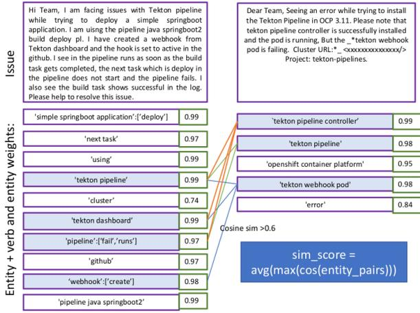
Figure 4: Example of similarity score calculation between two issue texts. The retrieved entities and the corresponding verbs are shown along with their weights, for the two issues. Connection between a pair of entities are shown by a line when the cosine similarity in the embedded space exceeds the value of 0.6. The final similarity score for the two issues shown in the example is 0.72. Sensitive information have been blocked.
