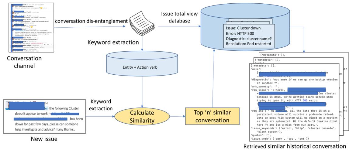
Figure 1: The framework of our proposed approach. Sensitive information have been blocked.
