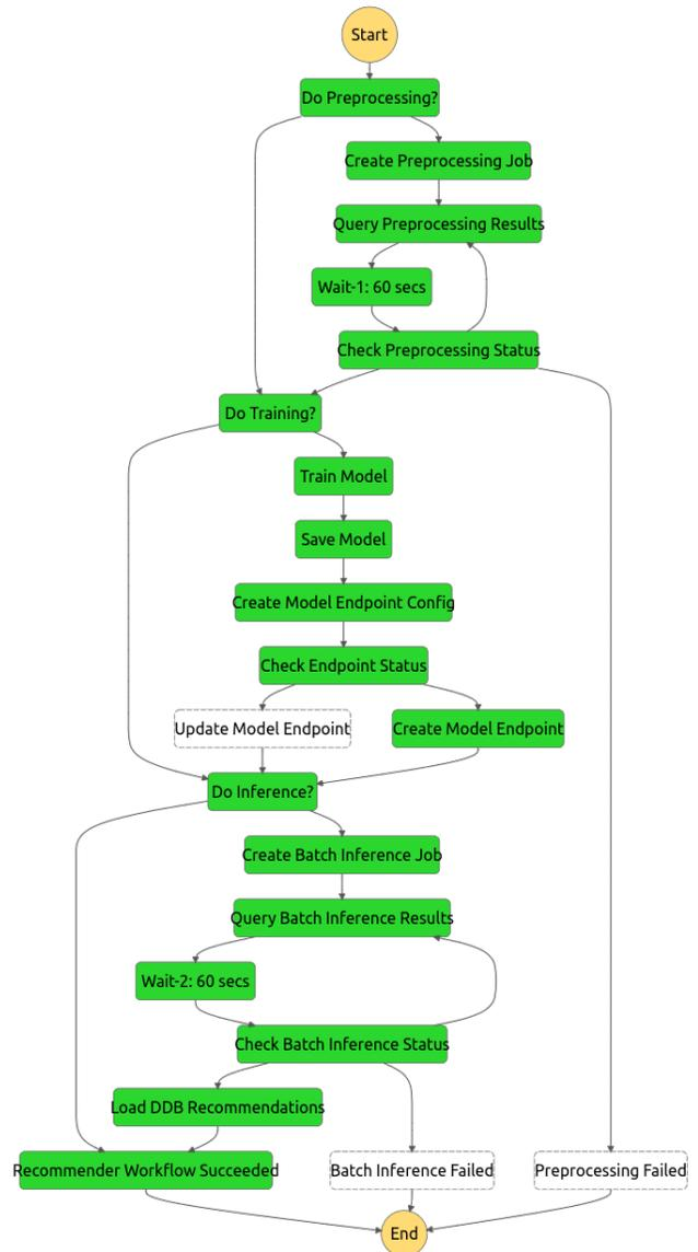
Figure 9: A successful execution of the workflow
